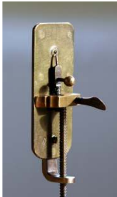
Figure 7-2. A reproduction of van Leeuwenhoek's microscope constructed in the modern era. Van Leeuwenhoek kept key details of his lens grinding process private, and a successful reproduction of the microscope wasn't achieved until the 1950s by scientists in the United States and the Soviet Union. (Source: Wikimedia .)
